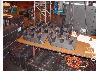
Figure 2.48 Radio communication is often critical when setting up remotes. Often, due to frequency coordination issues, the necessary radios will be rented in the city where the remote will take place.
