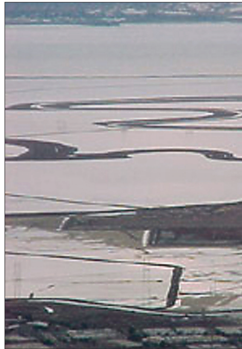
Figure 2.31 Microwave paths over water are often problematic as atmospheric conditions may refract the microwave signal and cause it to miss the receive dish.
