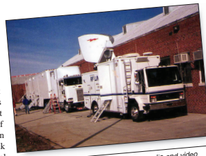
Figure 2.32 Ku satellite truck receives audio and video outputs from the production truck behind it and uplinks them back to the television station, approximately a 46,000-mile trip up and back down from the satellite, whether the station is across town or across the country. (Source: Tim Stoffel)
