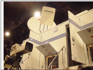
Figure 2.53 Hard camera rig outside combination production/ku uplink truck. This situation greatly simplifies planning and setup.
