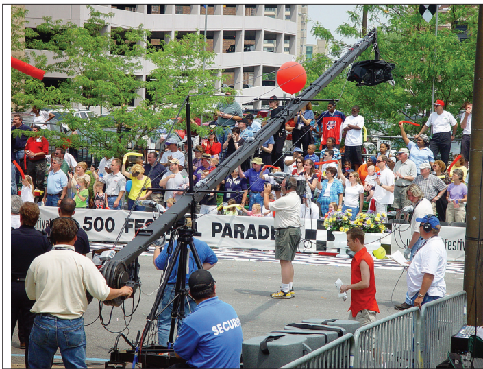
Figure 2.46 Camera mounted on a jib arm. The camera at the end of the boom is controlled (pan and tilt) via cables, which are controlled by electric motors run by the jib operator. Besides allowing the camera to get where a mortal alone couldn't, the jib arm also allows for sweeping camera moves in which the camera appears to fly over crowds and action.
