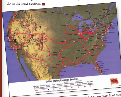
Figure 2.40 Many paths back to the station or network today are over fiber optic cable. The leading provider of fiber paths for television is Vyvx, which is part of Williams Communications. Many venues and television facilities have Vyvx terminal gear. The video and audio signals are converted to digital data for travel over the network. (Source: Williams Communications/Vyvx)
