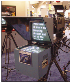
Figure 2.42 Often special equipment or appurtenance must be mounted on cameras such as this prompter system. Yes, some of the light from the prompter monitor does reflect into the camera lenses. So adjustments to the camera usually have to be made.
