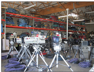
Figure 2.49 The types of cameras needed, either studio type (in foreground), which are also known as “hard” cameras, or handheld cameras (at rear and right of photo) must be determined. Also important is the lens that each camera will have. These studio cameras have 67:1 zoom lenses mounted. Most large
