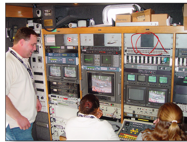
Figure 2.36 Inside compartment of a Ku uplink truck. This particular truck can also act as a small production truck, as it has a small video switcher (right bottom of photo) and mixer. The right three racks are for baseband audio and video. Baseband means the audio and video that has not yet been modulated onto a RF carrier. The right two racks take the audio and video and communications from/to the truck and turn them into RF signals for transmission up to a Ku satellite. This truck is equipped for both analog and digital transmission.
