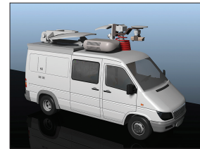
Figure 2.33 This is a combination Ku and ENG van. Rear dish folds up and is rotated toward the desired satellite. The front mast is extended up and its mast folds up and is pointed toward a microwave receive site. (Source: Wolf Coach)
